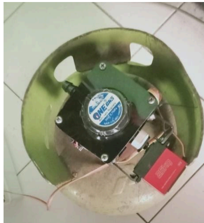
Figure 4. Top-view of sensor and servo motor testing
